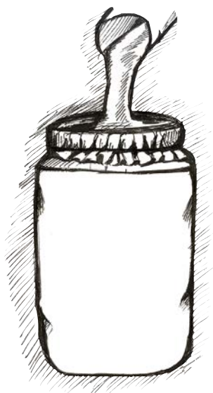
Cloth filtration for turbid water
