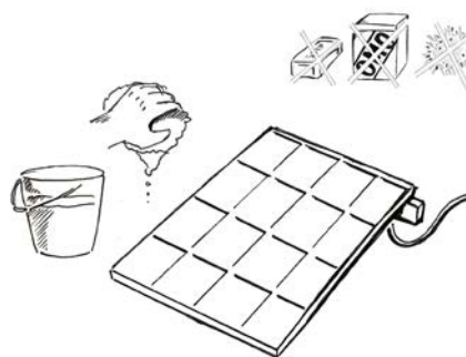
Clean solar panel with water and a cloth
