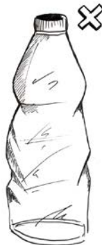
Bad bottles: heavily scratched damaged
