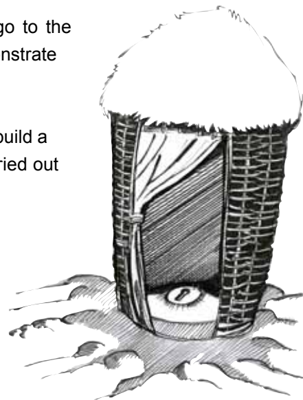
Single pit latrine
