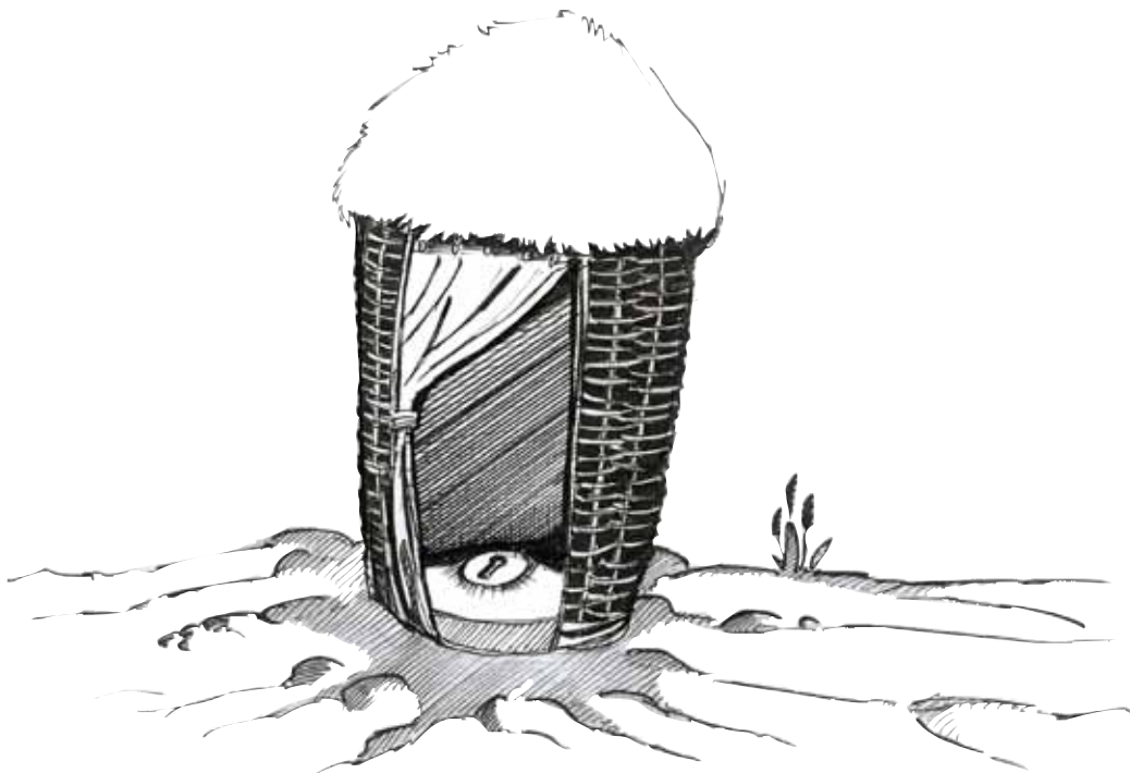
Single pit latrine
