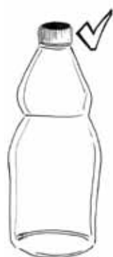
Good bottles: transparent unscratched not bigger than three litres
