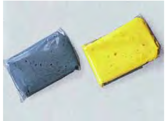
Fig. 184 Two-component, epoxy-resin putty
