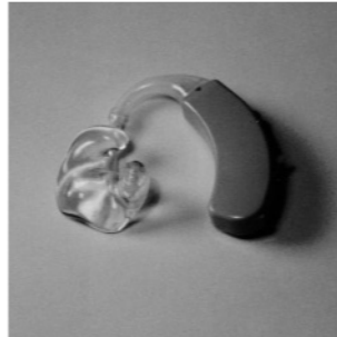
Earmould fitted wrong way to BTE hearing aid
