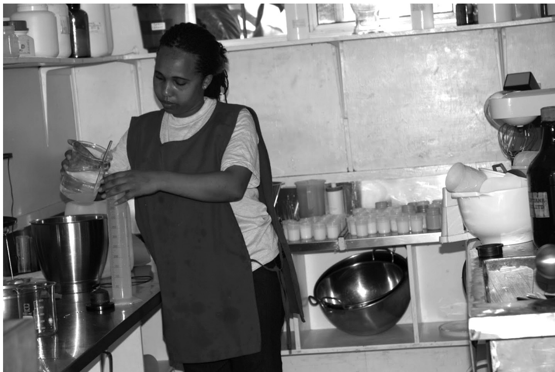
Figure 8.1. Using a graded measuring cylinder: transferring a solution prior to making up to volume
