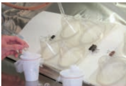
Figure 3. Cone bioassay of long-lasting insecticidal mosquito nets. Courtesy of Dr Vincent Corbel, Institut de Recherche pour le Développement, Montpellier, France. The holding board is held slanted at 45°.
