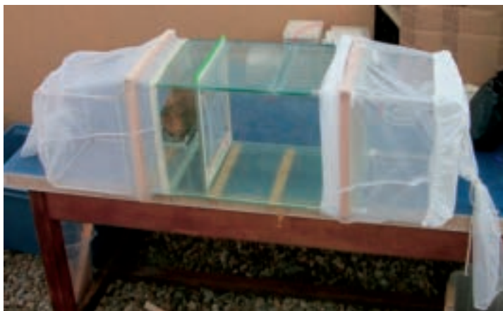
Figure 4. Tunnel made of glass for studying the efficacy of long-lasting insecticidal nets. Courtesy of Dr Vincent Corbel, Institut de Recherche pour le Développement, Montpellier, France
