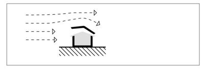
Figure 6.3(l) shows that a roof angled at  $20^{\circ}$ – $30^{\circ}$  receives the least wind stress.
