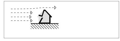
Figure 6.3(k) shows how low-pitched roofs receive a high suction and are likely to blow off as a result.
