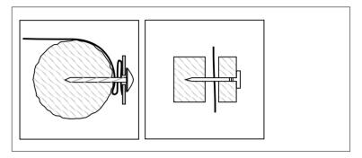
Using washers or thin pieces of wood as battens to attach the sheet can reduce tearing, but this should be done with care, because timber can have sharp edges.
