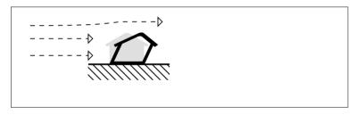
Figure 6.3(o) shows that a building that is shielded from wind, located at a safe distance to avoid trees falling on it, and built on a plinth, if correctly constructed, is well protected against winds and floods.
