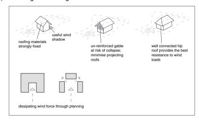
One of the primary mechanisms by which wind causes damage is 'uplift'. The roof should be tied down on to the walls, and these upward loads should then be transmitted all the way through to adequate anchorage in the foundations. It is important to ensure that the roof stays down when subject to the wind-uplift loads. Roof trusses need to be bolted to the load-bearing columns through incuts or straps. (See figure 6.3(i).)
