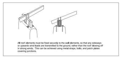
A well-anchored roof will prevent water entering during rain storms or tropical cyclones. If roof shingles (wooden tiles) are used, a simple preventative measure is to use eight nails per shingle, rather than four.
