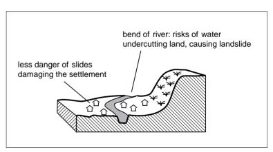
buildings Although solid foundations or raft foundations will improve stability on unstable soils (6.8.2), if the soil is moving in a landslide the building will still go with it, unless the foundation extends well below the region of soil movement.
