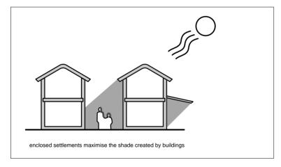
**buildings** Thermal mass in buildings should be ensured by constructing thick walls and insulating roofs, making them cool in the day and not too cold at night. In areas prone to earthquakes, the use of concrete blocks should be considered.
