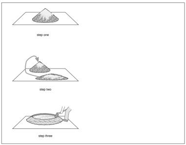
**Step 1:** start pouring the cement on top of the sand.
