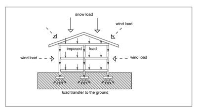
**types of load** The primary loads that all buildings must be able to carry or resist are as follows:
