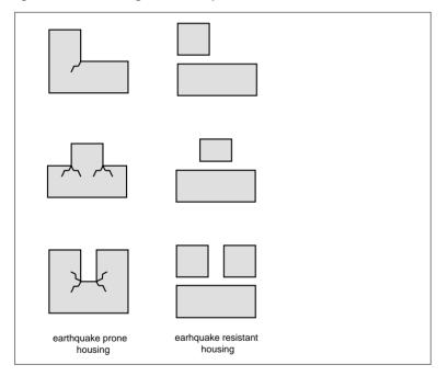
It is recommended that where a structure has to be built with a number of units, the units are connected through non-structural sections, and the buildings are structurally built of separate elements.
