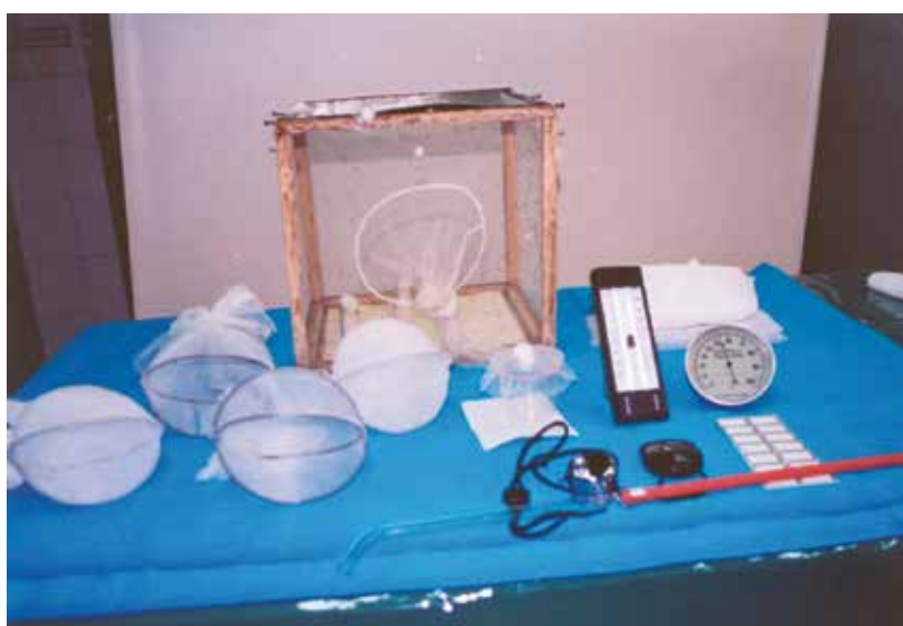
Figure An7.7 Composition of test kit using netting apparatus with wire frame
