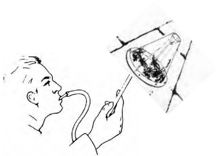
Figure An6.2 Releasing mosquitoes, using a straight aspirator, into the exposure chamber
