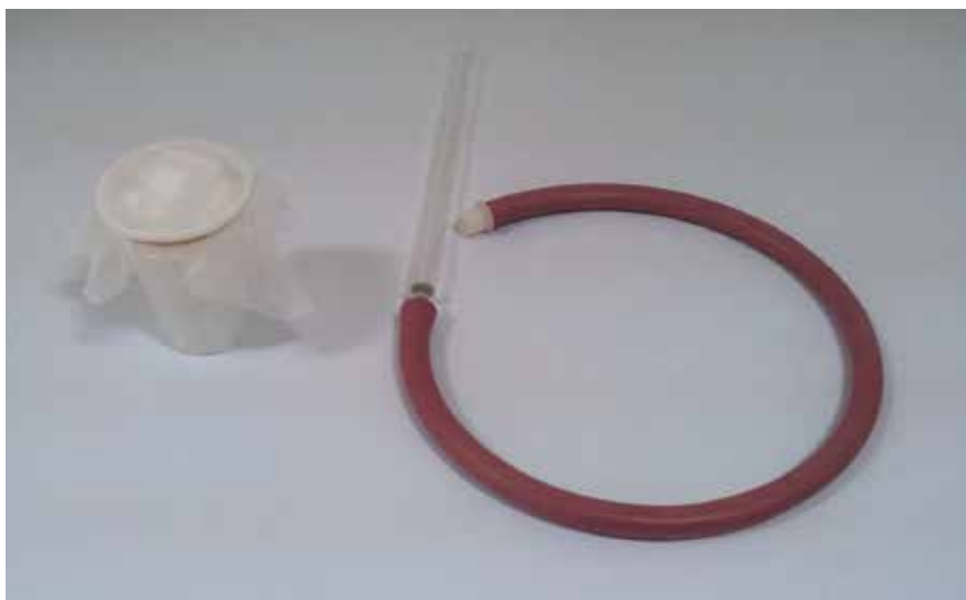
Figure 3.1 Sucking tube (or aspirator) and paper cup for hand collection of adult mosquitoes
